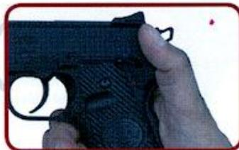
8 Push the Safety downwards to the "Off Safe" position. Pull the trigger to fire the gun. When finished shooting, remember to put the Safety back on "Safe"
