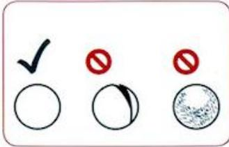
Always use precision 4.5mm pellets for this Airgun. Never use any used or damaged pellets.
