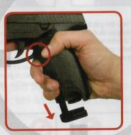
**2** Push the Magazine Release Button and pull out the magazine.
