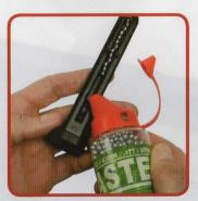
5 The Airgun is now ready to be loaded with 4.5mm steel pellets. Remember to release the pellet hatch after loading the pellets.
