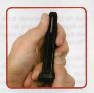
4 Pull and hold down the pellet hatch until it is locked in position.
